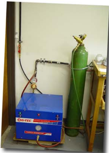
Torch Boosters can be installed next to jewelers' benches - they are quiet and do not require any special site preparation
