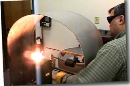
High-pressure natural gas easily melts platinum and improves the quality of platinum casting
